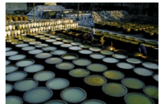
The process of making Shaoxing yellow wine. (Photo by Xie Guanghui, provided by image library of Hong Kong China Tourism): Steaming rice (1) → Cooling (2) → Airproof fermentation (3) → Adding water (4) → Distillation
