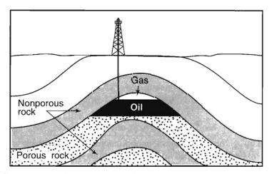
Look at this diagram. Here is an example of an anticline. As you can see, the oil is trapped under a formation of rock that resembles an arch. In this anticline, the petroleum is trapped under a formation of nonporous rock with a gas deposit directly over it. This is fairly typical of an anticline.
