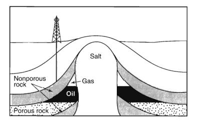
Now, let's look at a diagram of a salt dome. This salt dome shows how a cylinder-shaped salt deposit has pushed up through a layer of sedimentary rocks, causing them to arch and fracture. The oil deposits have collected along the sides of the salt dome.
