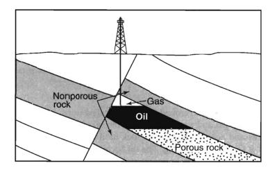
Finally, I want to show you a fault trap. This diagram represents a fracture in the Earth that has shifted a nonporous rock formation on top of a porous formation. Remember, as in all traps, the oil is collected in the porous rock and trapped underground by the nonporous rock.
